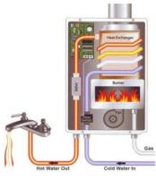
Most tank-type water heaters are anywhere from 60% to 67% energy efficient. Tankless water heaters are 90% to 98% efficient. So the savings are twofold, higher efficiencies and no stored water being kept at 120 degrees, whether you are using water or not. Another byproduct of high efficiency is reduced green house gasses contributing to cleaner air and better quality of life for all.
